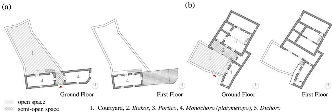
Figure 4 Typical rural dwelling typologies (a) *Monochoro* typology with *portico* in linear shaped configuration (b) *Dichoro* typology with *iliakos* in L-shaped configuration.
