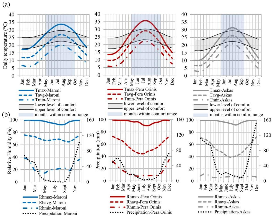
Figure 3 (a) Mean minimum, average and maximum air temperature, comfort range limits ( $\pm 3.5$ , 80% acceptability limits) using Ashrae Standard 55 ( $T_n = 17.8 + 0.31T_{avg}$ ) and months within comfort range (b) Mean minimum, average and maximum relative humidity and average monthly precipitation at Maroni, Pera Orinis and Askas villages respectively.
