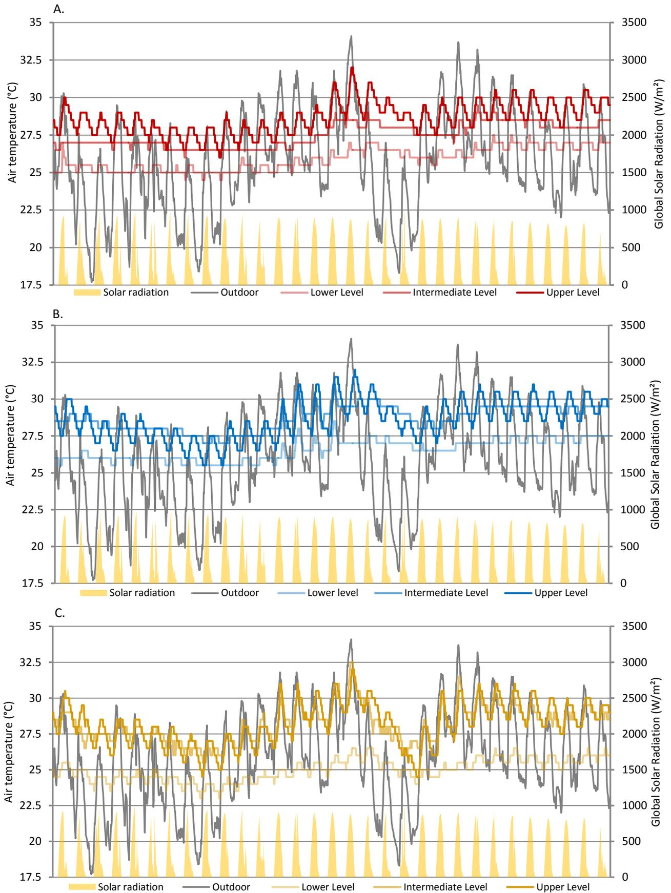
**Figure 2.** Profile of onsite air temperature measurements between 1st and 31st of August for A. Case Study A, B. Case Study B and C. Case Study C
