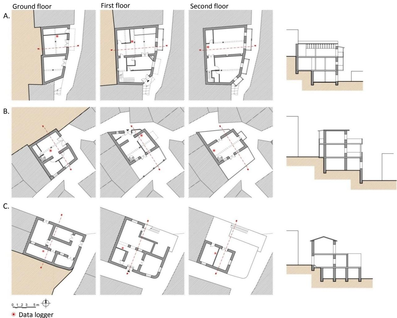
**Figure 1.** Plans and sections of traditional buildings showing the spaces where onsite air temperature measurements were carried out: A. Case Study A, B. Case Study B and C. Case Study C
