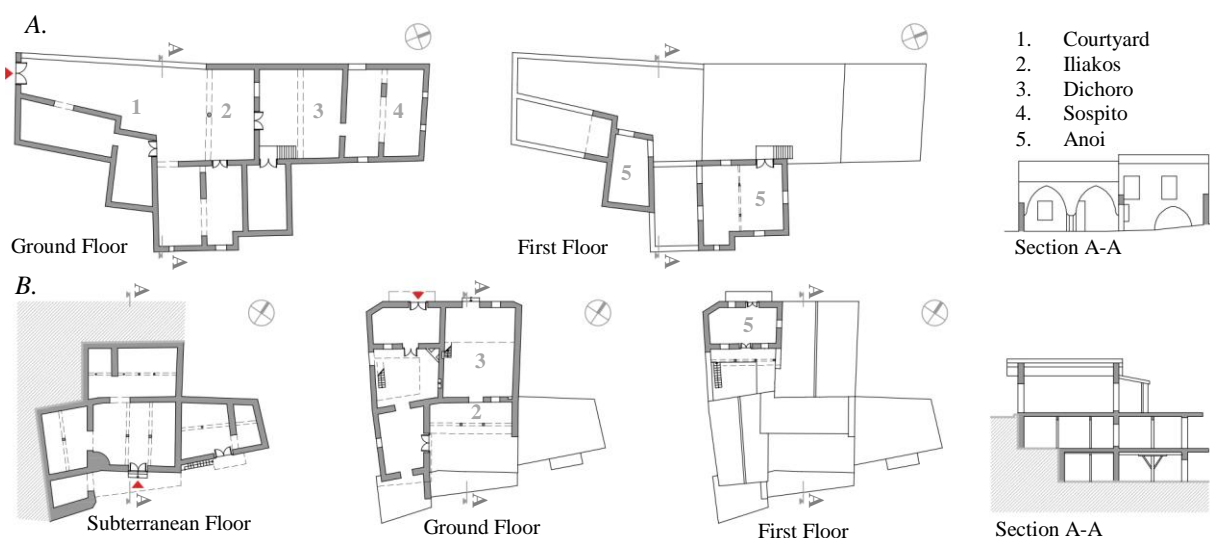
Figure 2 A. Typical plan layout and section at A. Pera Orinis settlement and B. Askas settlement
